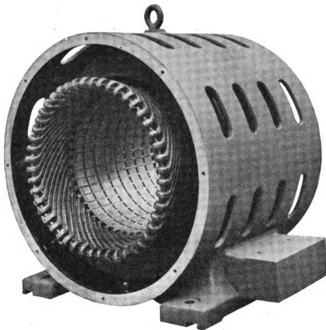
FIG. 119.—Lattice-type coils on the stator of an induction motor.
